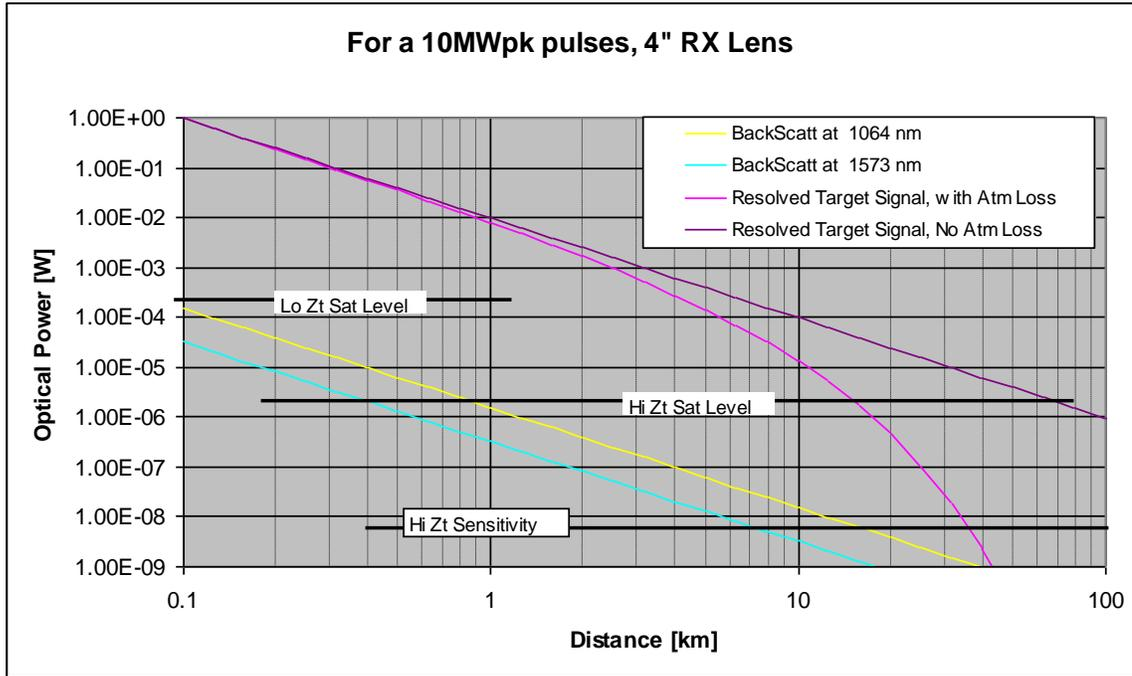
**Figure-1: Signal and Backscattering power levels**
