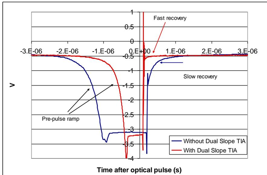
Figure-9: Overload recovery signal with  $320\text{ kW}/\text{cm}^2$  pulses, 4 ns FWHM
