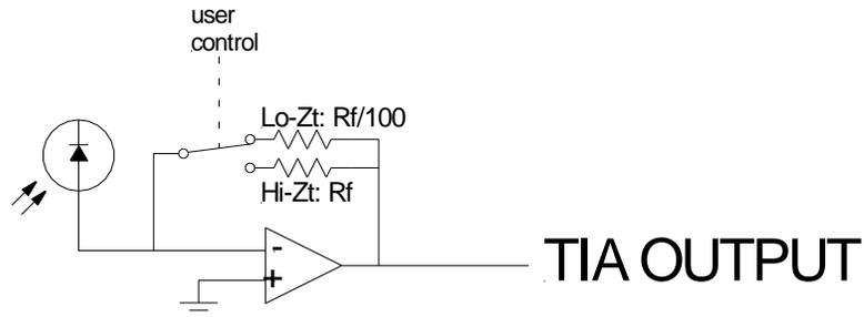
**Figure-2: Proven switchable Rf**
