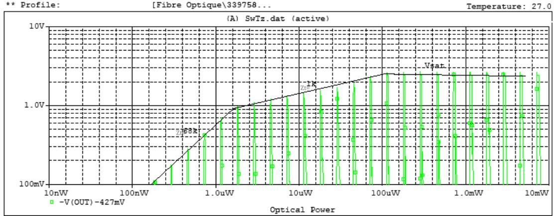
Figure-7: Dual Slope Receiver
