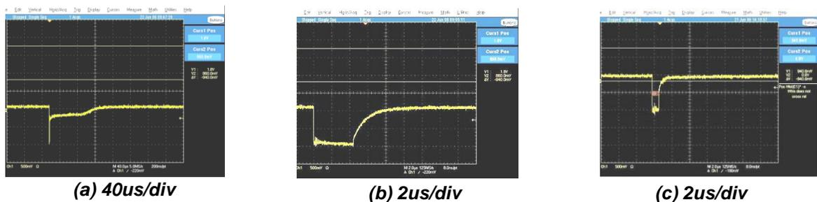
Figure-6: APD recovery time evolution @ 332kW/cm<sup>2</sup>.
