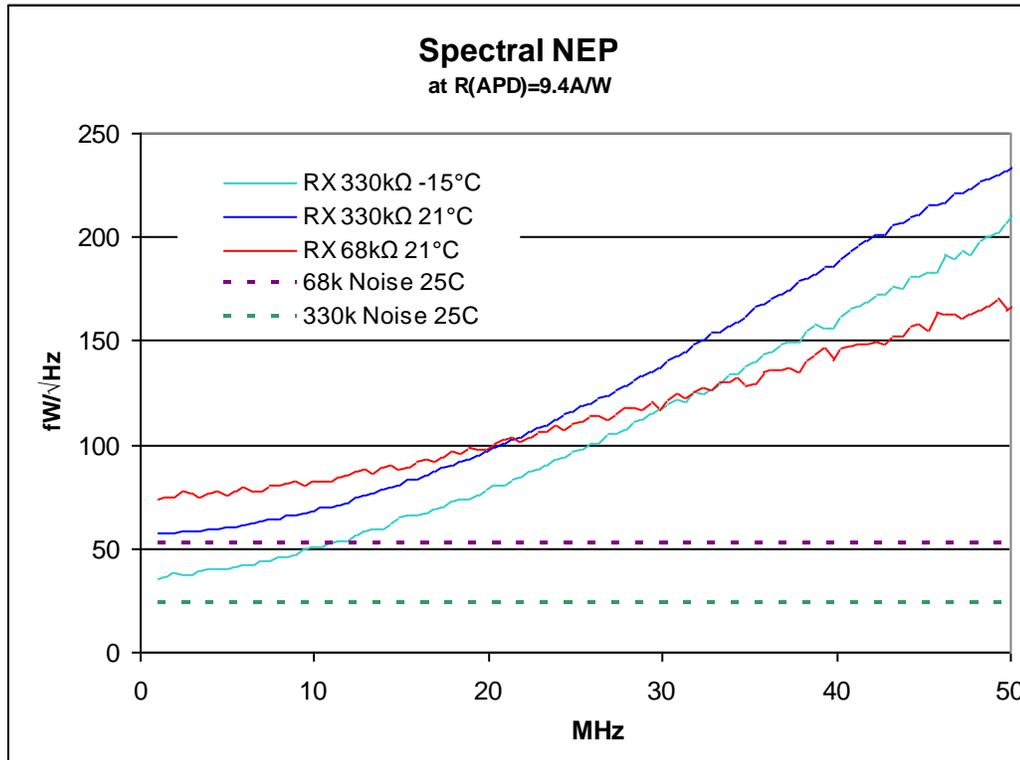
Figure-10: Spectral NEP comparison with 68k $\Omega$  and 330k $\Omega$  feedback resistors.
