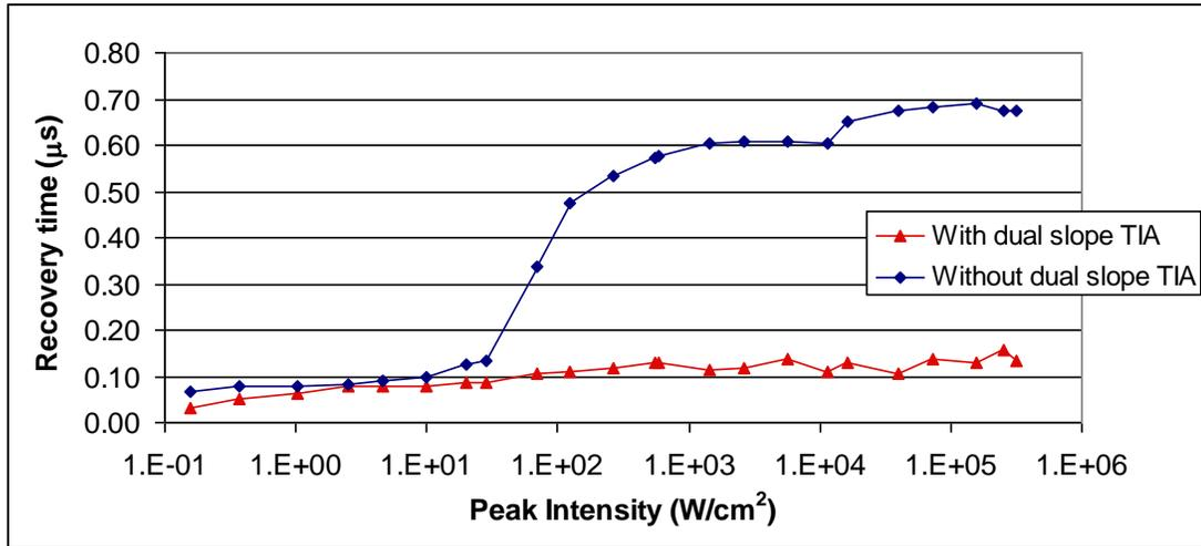
Figure-8: Overload recovery time to 200 mV with  $320\text{ kW}/\text{cm}^2$  pulses, 4 ns FWHM
