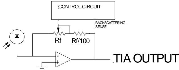
**Figure-3: Continuous Auto switching Circuit**
