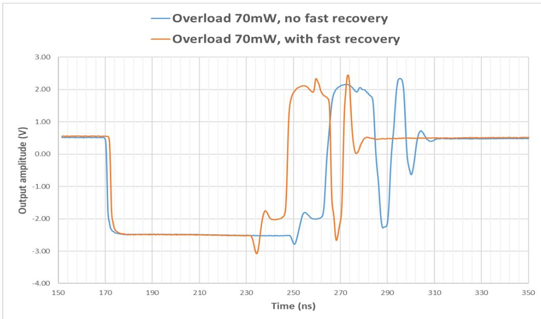
**Figure 2: Fast recovery circuit reduces the recovery time by 20-25ns (14%)**
