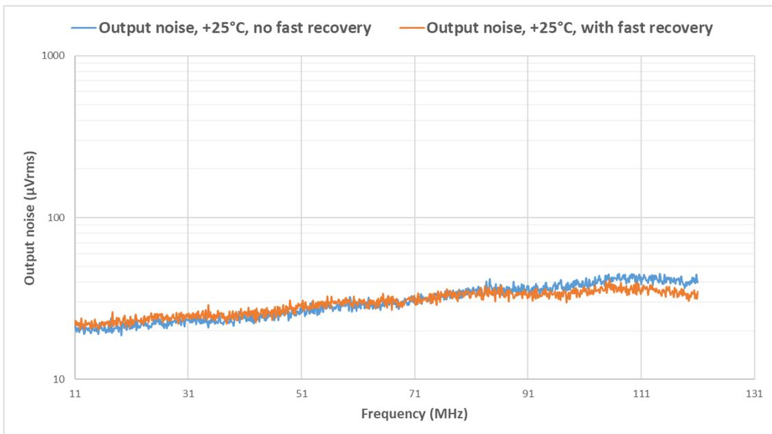
**Figure 3: APD receiver output noise at ambient temperature, with and without fast overload recovery**
