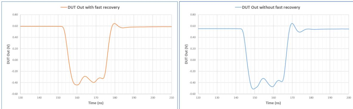
**Figure 4. 1V output swing in linear mode, showing rise/fall time of 3.2ns and 2.8ns for receiver with and without fast overload recovery circuits.**
