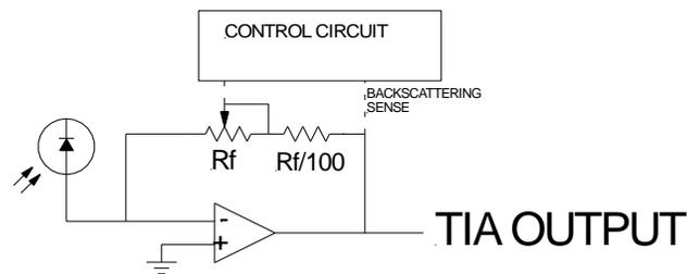
**Figure 1 - Continuous auto switching circuit**
