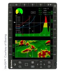
Real-time weather, moving map, synthetic vision with tactical data overlay
