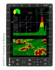
Real-time weather, moving map, synthetic vision with tactical data overlay
